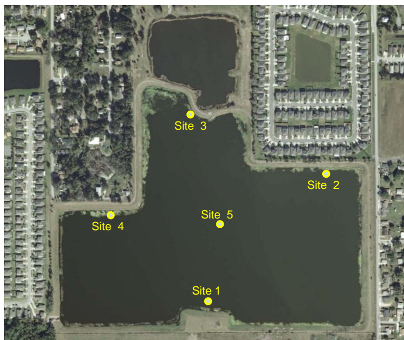
Figure 2-8. Seepage Monitoring Sites in the Club II South Pond.
